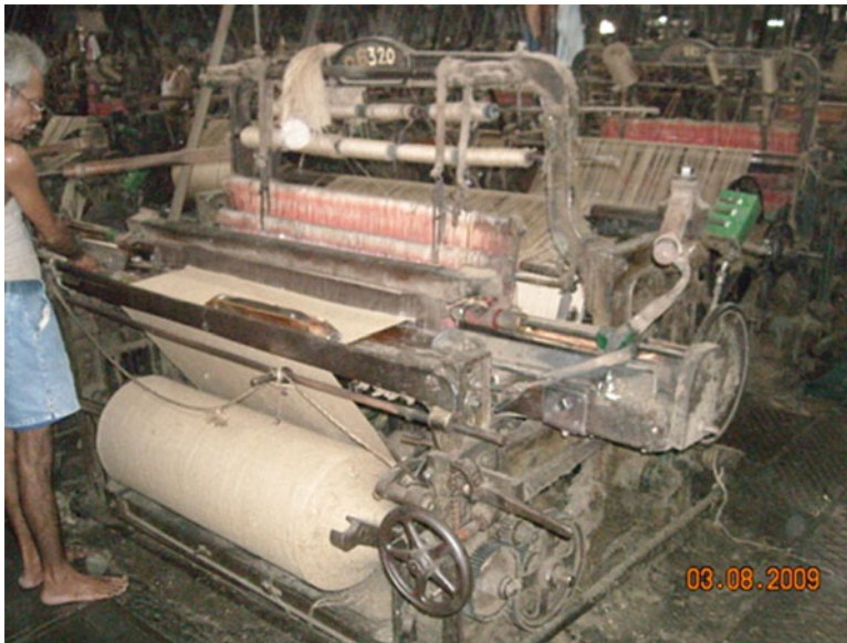
Fig. 2.4 Manufacture of jute fabric in loom
