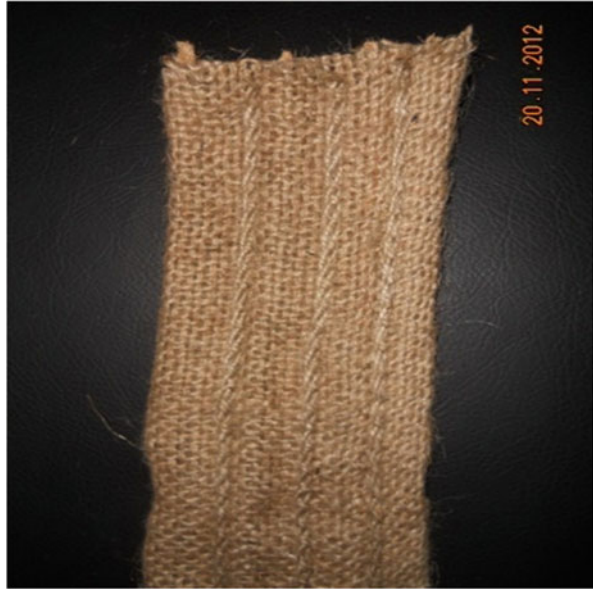
Fig. 10.1 Typical PVJD with coir wicks
